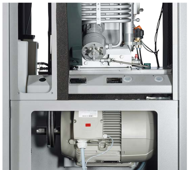
Interior view of VERTICUS: Adjustment of the V-belt is not necessary because of the vertical format and suspended motor mounting.
